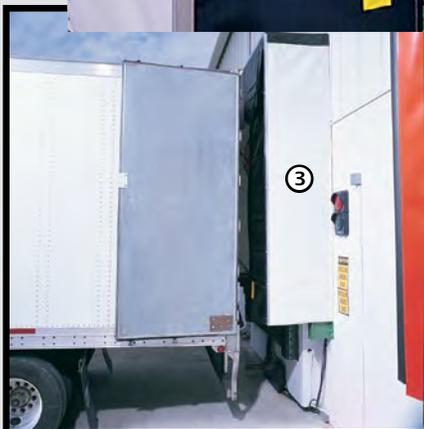
As the trailer approaches, if off-center trailer contact occurs, the FlexFrame moves upward and back to prevent costly damage to the wall and shelter. After the trailer leaves, a gravity-biased design returns the frame to its original position.
