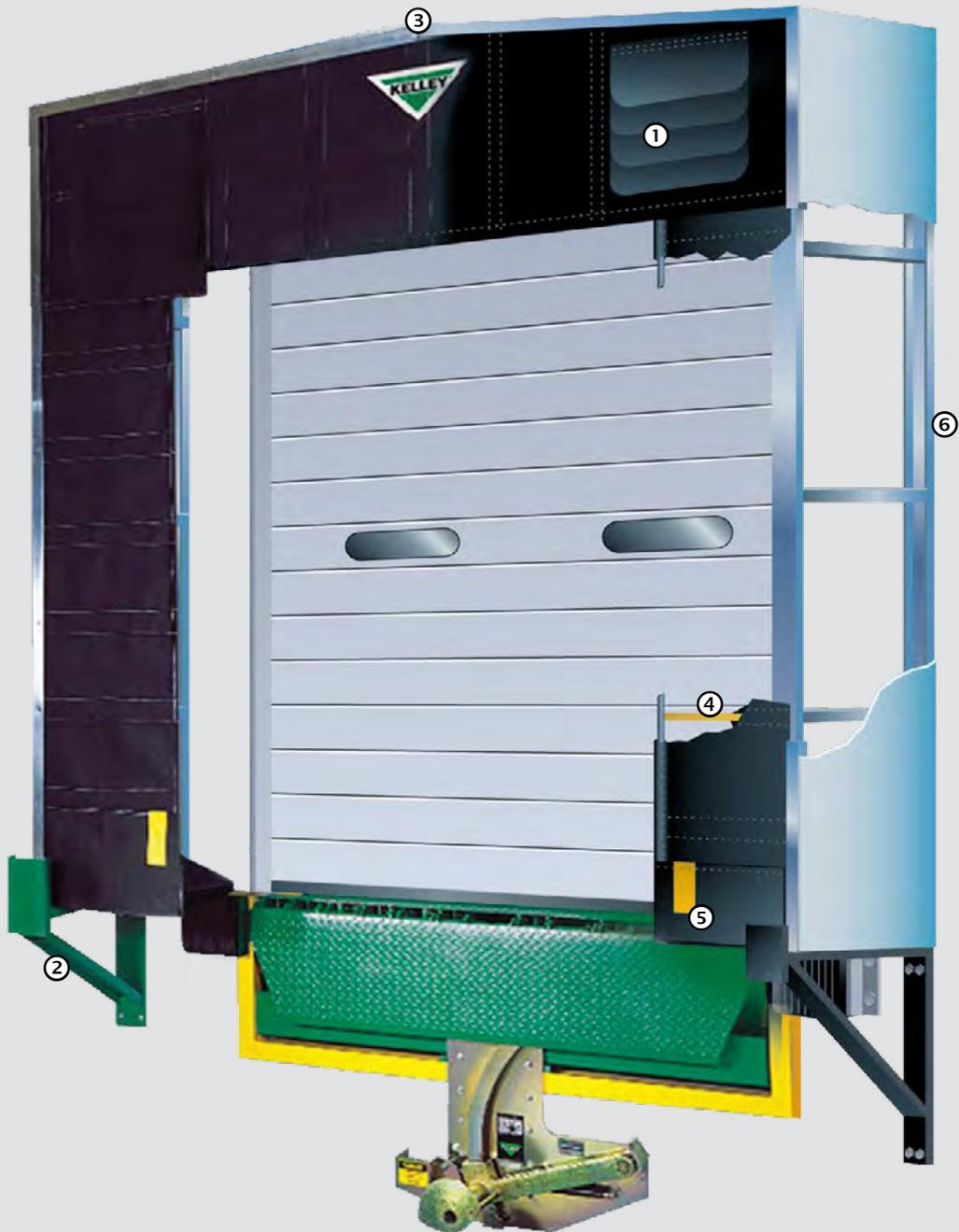
① *Overlapping wear pleats sewn to the head curtain provide extra resistance against the sharp corners of the trailer, extending the life of the shelter.*
