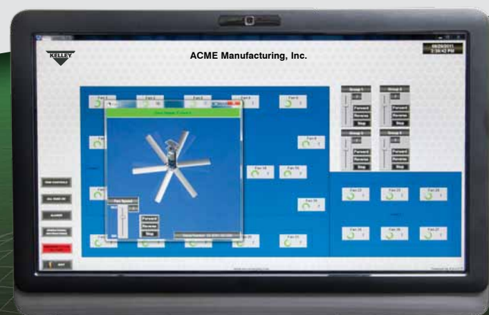
Dialog box for individual fan provides access to direction and speed settings for a specific fan.
